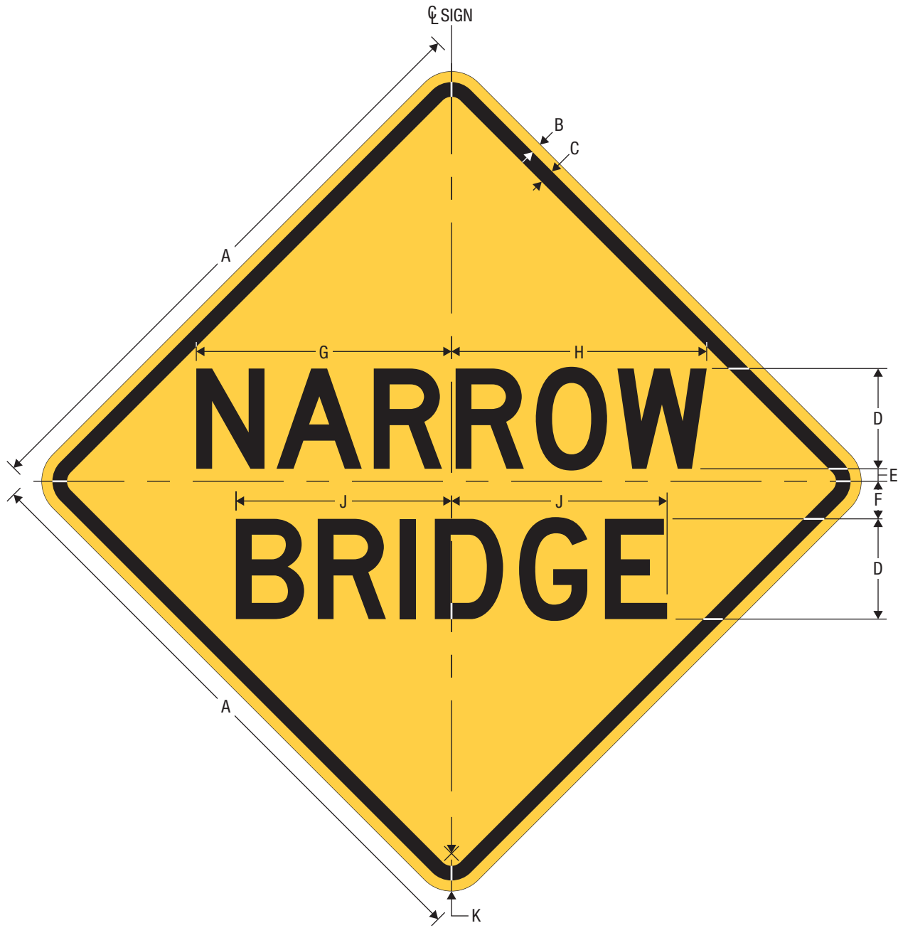
W5-2 NARROW BRIDGE
