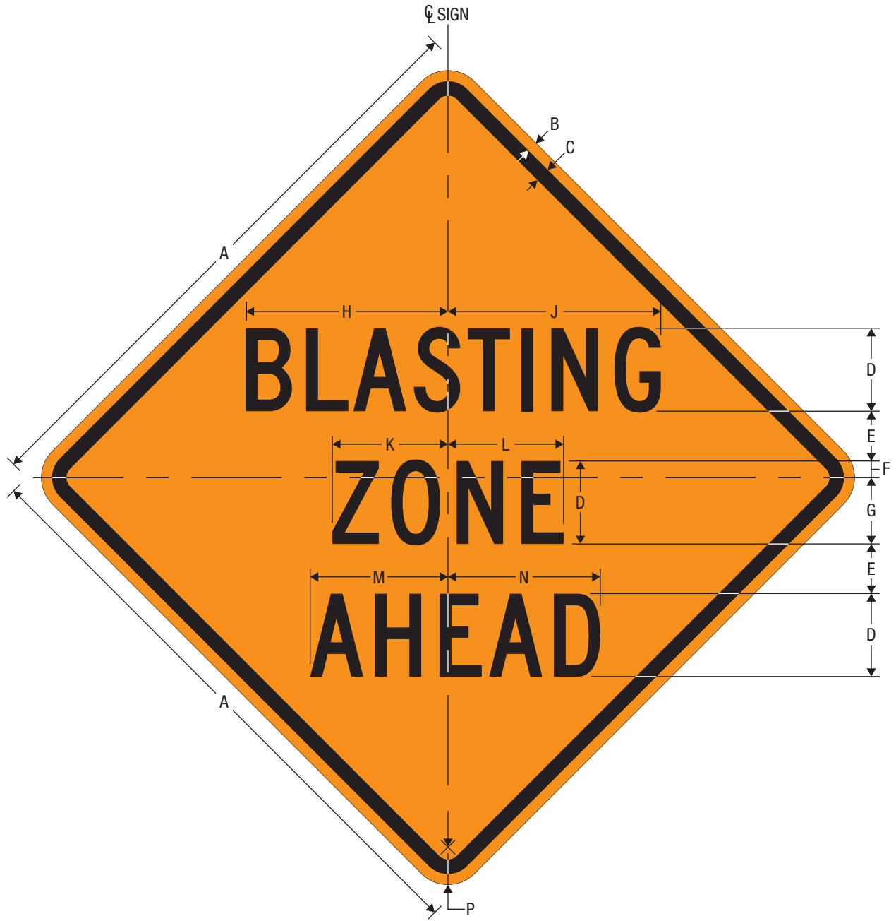
W22-1 BLASTING ZONE AHEAD
